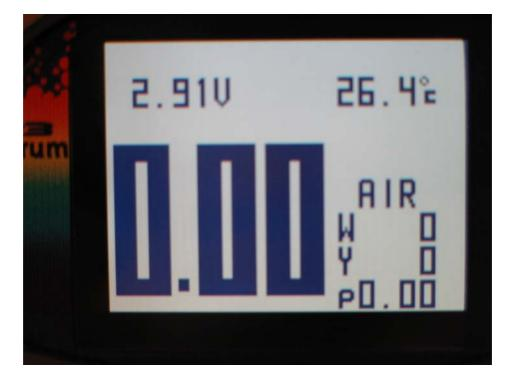
• X mode the dry screen saver is displayed with PO2 in large numbers in the bottom left of the screen, HP contents and PO2 on the bottom right and current battery voltage and temperature along the top line.
