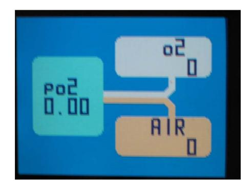
• When in N mode this is the screen saver display you will see, this displays a PO2 reading and O2 and diluent tank pressures. When viewed with the colour screen option the tank pressure colours correspond to the coloured tapes on the HP sensors, white for oxygen, yellow for diluent.
